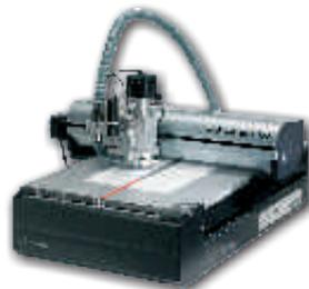
Mill and drill the board layers on a ProtoMat H100.
